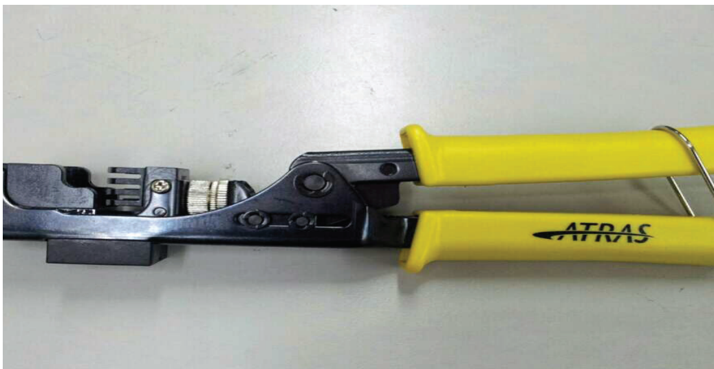
Punch Down Tool for 180° Cat 5 & 6 Atras Jacks
